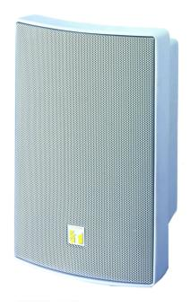
The BS-1030W is a small, 2-way bass-reflex type speaker featuring a wide frequency range suitable for use for announcements and music playback. The BS-1030W can be used for both high-impedance and low-impedance applications. The speaker's splash-proof construction permits it to be installed under the eaves where the speaker is not directly exposed to rain.
