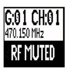
Use this to turn on a transmitter without interfering with the RF spectrum.
