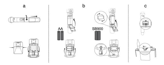
The transmitter runs on two AA batteries or a Shure SB900 series rechargeable battery. Use the included AA battery adapter when using batteries other than the Shure rechargeable battery.
