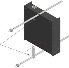
Cut outs and mounting tab may be used to suspend the unit above the ceiling using hanger wire.
